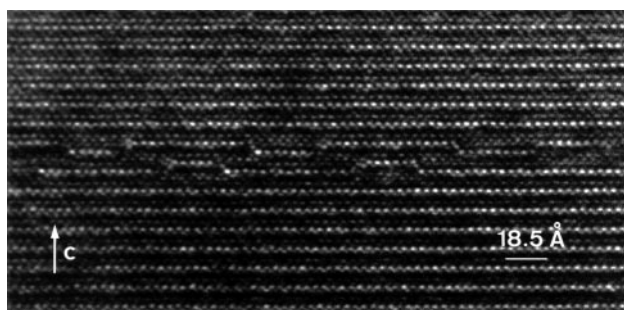
Fig. 4 [100] HREM image for \text{Li}_2\text{SrNb}_2\text{O}_7 showing domains of an n=3 member interleaving the parent matrix.
